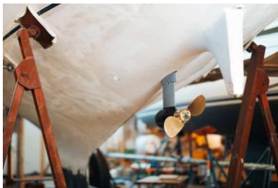
The electric engine is built into the pod drive under the hull. The folding propeller will drive the boat as well as charge the batteries generating “hydropower” while sailing. Photo: janajulian.com
