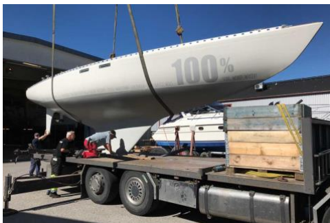
The Smaragd leaving the shipyard for launch some days ago. The electric engine in the pod drive is simply placed under the hull and the folding propeller will be used to charge the batteries while sailing.
