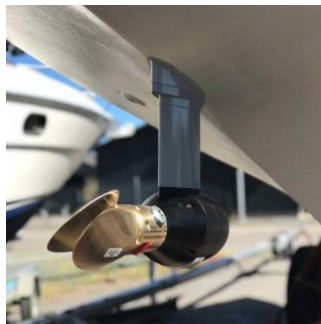
The Smaragd leaving the shipyard for launch some days ago. The electric engine in the pod drive is simply placed under the hull and the folding propeller will be used to charge the batteries while sailing.
